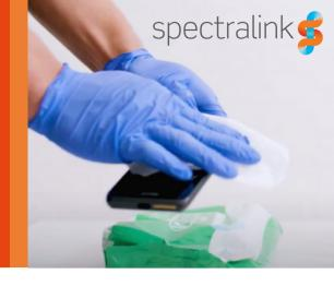
Spectralink's Versity Series smartphones are made with medical-grade resin designed to hold up to repeated cleaning from many of the standard antimicrobial surfactant detergents used in healthcare settings to clean and disinfect medical equipment.
